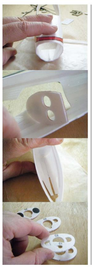
Take the fuselage and pre-bend the creases on the inside of the fuselage. Place a small piece of wax paper on your work surface so your parts won't get glued down. Hold together the edges on the front bottom so the first panels are flat to each other. Apply some CA glue to the seam and hit it with some accelerator. Once it hardens, you should hit the bottom side with accelerator as it was covered by the wax paper and may not be cured yet.
