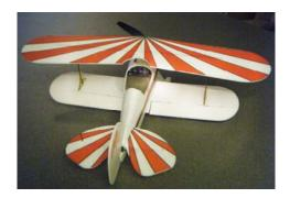
With a 120mah battery, the Center of Gravity should be just behind the leading edge of the lower wing. It is preferable to trim with weight, but you can tweak the ailerons for trim if you are not using an aileron servo. Try to be conscientious of when your battery will run dry. It really does not have much of a glide ratio and will come down like a rock, making dead stick landings a trick.
