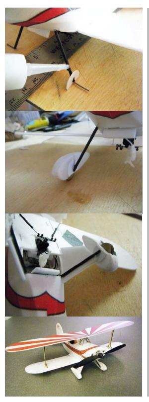
Set the plane on a flat surface (preferably with wax paper (not shown) so it doesn't get glued to the flat surface). Set the wheel pants bushing on the landing gear strut as shown so it is straight and vertical. Apply a small drop to the landing gear strut and let it drip down to the bushing. Hit it with the accelerator and this will tack it in place.
