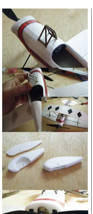
Glue on the center wing struts to fuselage.
